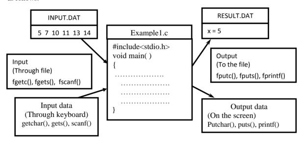
After a file is opened, we can read data stored in the file or write new data to it depending on the mode of opening. C standard library supports a good number of functions which can be used for performing I/O operations. File I/O functions are broadly classified into two types.
