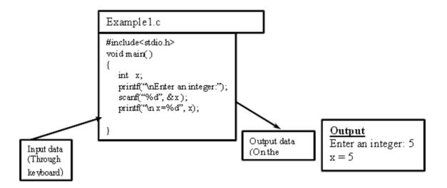
In the above program the data that is input through keyboard and that is output on the screen is temporary, because the data is stored in main memory. So whenever the application is closed or the system is switched off the entire data on main memory is lost. So it is not possible to see the data in future. Since these I/O functions use keyboard and screen, these functions are console oriented I/O functions. Using these functions it is not possible to store data permanently in the system.
